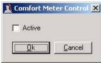
Used for managing the attached comfort meters (if any). If the checkbox is checked the comfort meters will be active, and operate according to there *mode*-settings.
