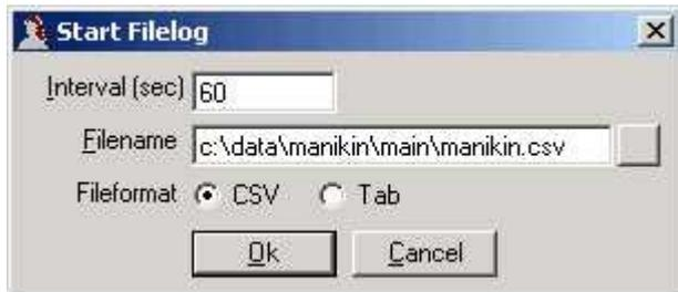
The filelog saves data in to a file. Data is printed for all body parts. Filename gives the name of the data file. Interval specifies the time-interval in seconds for saving the data. The data will be a mean-calculation over this period. Fileformat specifies whether data are saved in Comma Separated Values (CSV) format or tabulator separated format. Both format should easily be imported by fx spreadsheets and database programs. The decimal settings follows the standard Windows settings.
