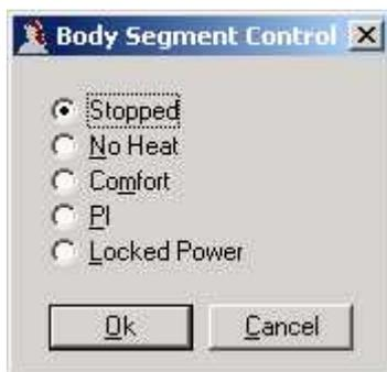
Used for managing the control method of the manikin. No Heat / Comfort / PI / Locked Power specifies the actual method for controlling the fired power (for a description of the different types of control available refer to [Appendix - Methods of control](#)).
