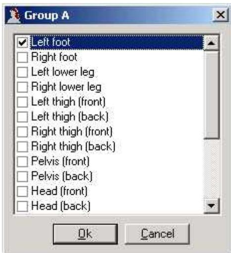
Group A and Group B indicates if a specific part of the body is to be included in the mean calculation of temperature and power value for group A and B respectively. The mean calculation is performed as a weighted mean according to the areas of the different parts of the manikin.
